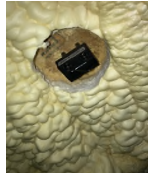
Figure 1 and 2 A portion of the foam was removed, the monitor was attached to the bottom of the roof decking, covered with plastic and the spray foam was reapplied to
